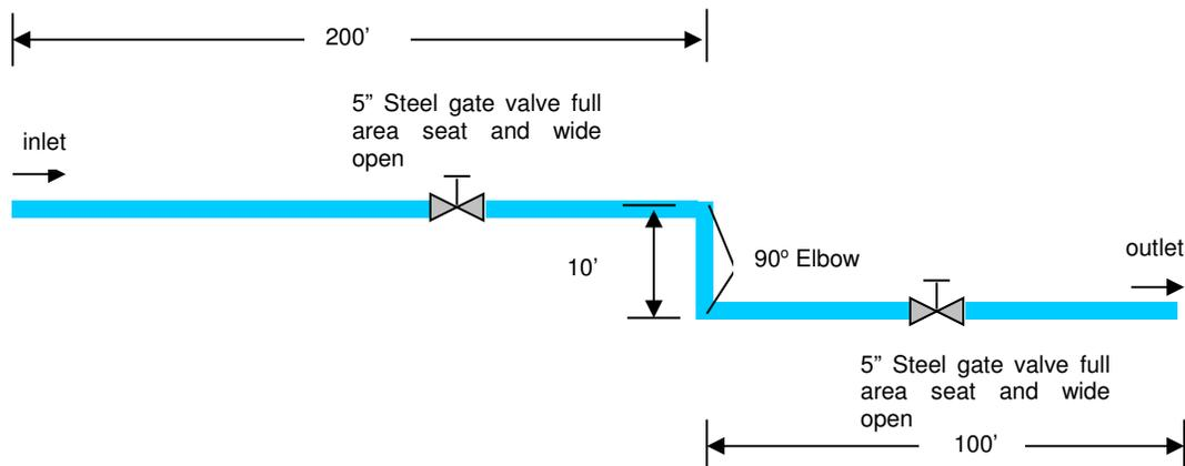
Find velocity in ft/s of the flow and the pressure drop in system from inlet to outlet and in format psi/100ft.
