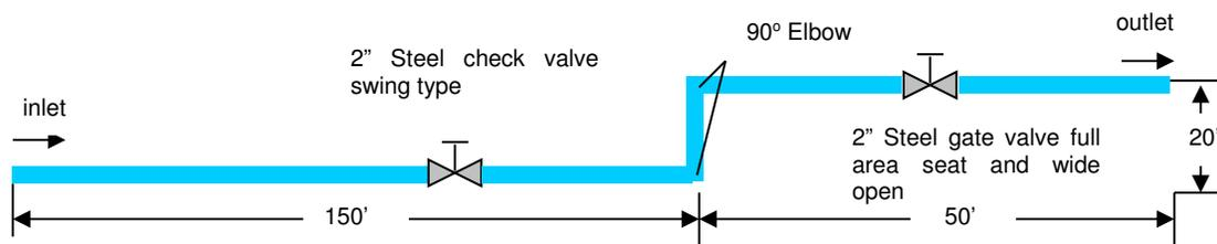
Find the velocity in ft/s and the pressure drop from the inlet through outlet in lb/in<sup>2</sup> and pressure drop in psig/100ft.
