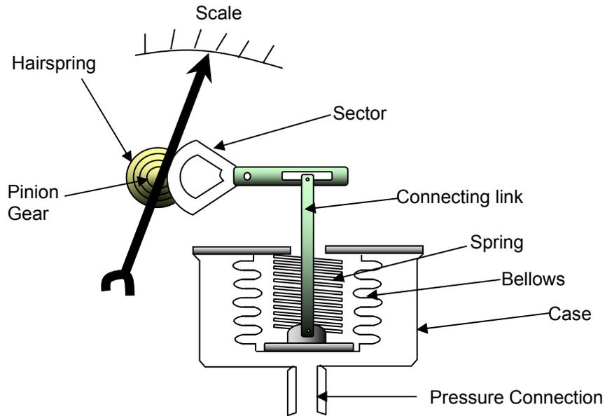
Figure 5: Spring-Loaded Bellows
