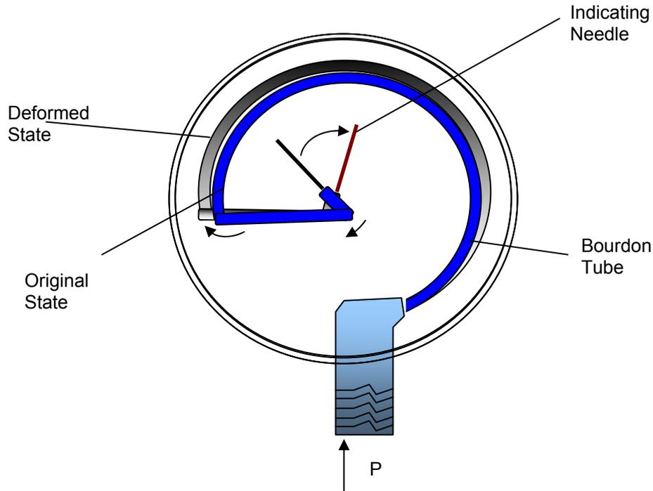
Figure 4: C-spring Bourdon-Tube Pressure Gauge
