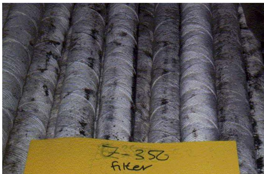
Figure 2 : Used Cartridge Elements
