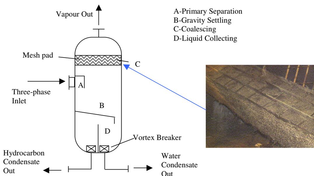
Figure 3 : Compressor Second Stage Suction Drum
