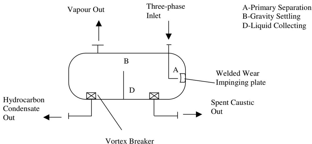
Figure 4 : Spent Caustic Deoiling Drum
