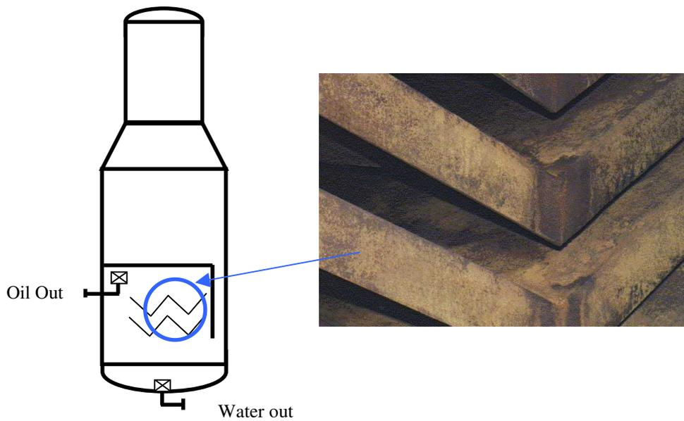
Figure 1 : Chevron-type Plate Baffles
