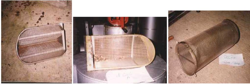
Figure 8 : W-shape, V-shape and Cylindrical T-strainer
