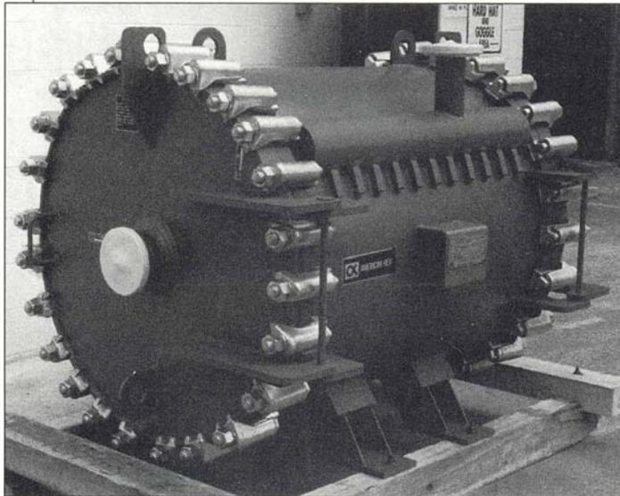
**The compact size of the spiral heat exchanger means no additional space is necessary if covers must be opened for cleaning.**
