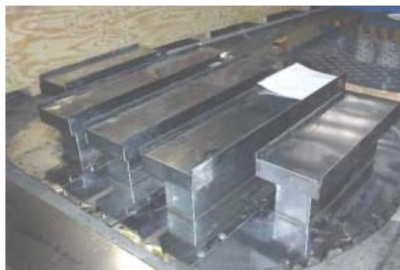
Figure 4: Picture of a Sulzer Chimney Tray
