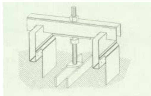
Figure 7: Schematic of New Distributor Support Plates
