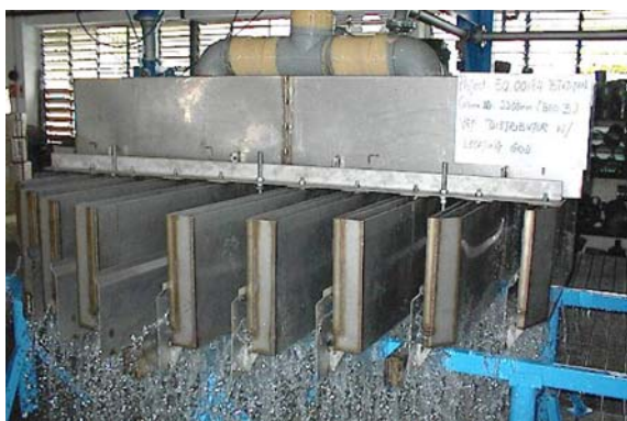
Figure 8: Picture of dual compartment distributor being tested at Sulzer Test Rig in Singapore
