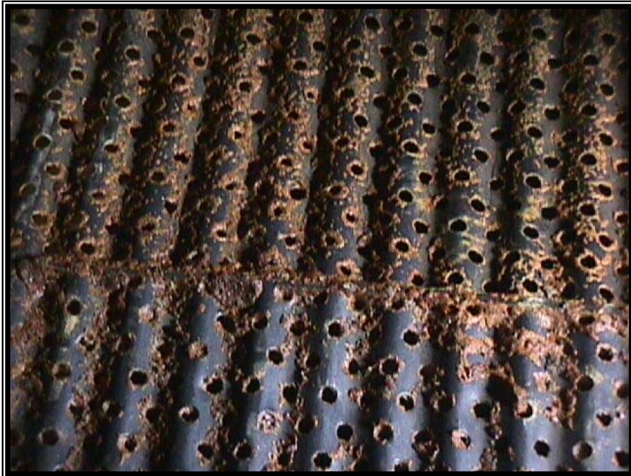
Example of Less Fouled Dual Flow Tray
