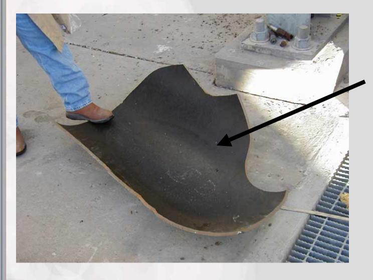
30" cold flare drum overhead line failure due to brittle fracture
